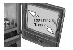
unscrewing the retaining tabs, taking care not to damage the fireproof rope seal. The replacement glass should be carefully placed against the seal and the retaining tabs re-tensioned. Take care to tension these evenly or there is a risk of breaking the new glass pane.
