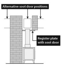
Horizontal register plate with top flue connection
