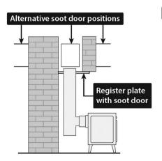
Horizontal register plate with rear flue connection
